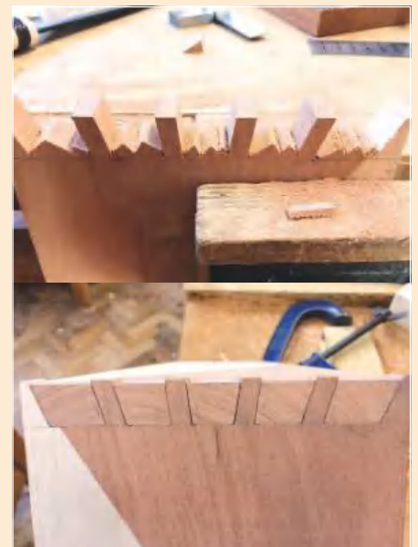
▲ Pic.20 I now had to measure and draw up the dovetails. In fact, I started to cut out the pins first rather than the tails, using a Veritas dovetail saw. I did try a pull saw but the Veritas made a cleaner cut and I found it easier to handle. After cutting, I filed down the saw marks to make the pins and tails fit even smoother. I was really pleased with how they turned out
